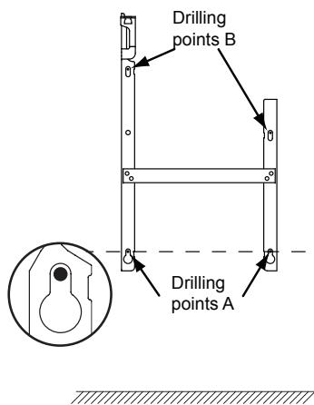
Drilling points **A** show the position for the lower fastenings.
