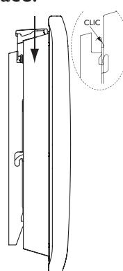
To unlock the device from the hanging frame, take a flat-bladed screwdriver and **push the slider towards the wall**.
