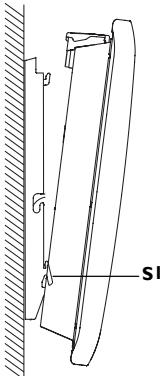
Pivot the device upwards and lift it to position it on brackets **S2**.
