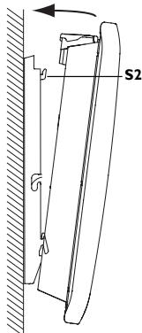
Lower the device onto the hanging frame. A click tells you that the device is fastened and locked in place.
