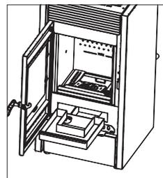
You can regulate the door adjustment in function of the progressive worn out of the seals through the screws that you will find on the stove frontal, by tightening and loosening these screws you will get the right adjustment of the door. (see drawing D10.4)
