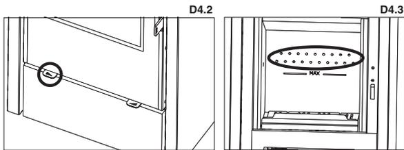
This control is placed at the bottom right side of the stove's door and the movement is done from left to right. The larger side of the triangle corresponds to the larger air inlet.
