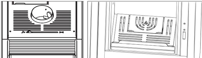
Primary air and double combustion regulations placed in the lower part of the stove door must be completely closed.
