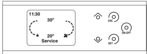
Please, bear in mind that the stove could need to be cleaned before this 1500 hours established by default or even after them. This depends on the quality of the fuel used, the smoke installation, and the proper regulation of the stove.
