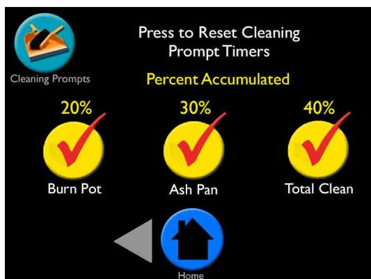
The Cleaning Prompts screen displays the percentage of time that has accumulated since the last cleaning. When it reaches 100%, you will get messages on the home screen to perform that specific maintenance. Press the checkmark on the home screen to reset. Resetting maintenance sets it back to 0% and tells the control to start calculating until the next cleaning is needed.
