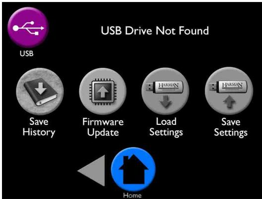
The USB screen displays actions that use the USB jump-drive port on the side of the EASY Touch Control. **Please Note:** The USB port **is not** a charging port for smart phones, tablets etc.
