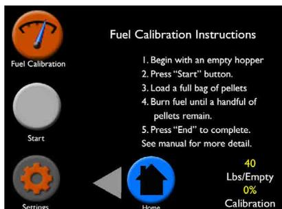
Fuel Calibration should be done for the most accurate fuel gauge and usage. When used in conjunction with the Hopper Fill screen (requires indicating when you add fuel. See Page 21), the Low Fuel Warning appears on the home screen at the most appropriate time.
