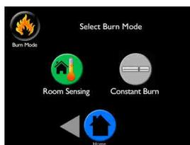
**Disabled and Constant Burn mode:** The stove must be lit in Automatic and then switched to Disabled. The stove will operate at your selected constant burn setting. The unit will not shut down unless the On/Off icon is touched or if the hopper runs out of fuel.
