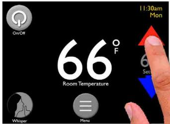
**Use the up and down arrows to set desired room temperature**
