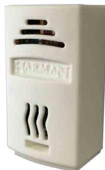
The wireless room sensor is powered by two “AA” batteries. If the batteries are low, you will receive a message on the home screen reminding you to change the batteries. If the batteries are exhausted, the home screen will tell you to replace batteries in wireless room sensor. If the batteries are exhausted, the unit will use the backup sensor to continue heating your home based on the temperature detected by this sensor located at the back of your unit.
