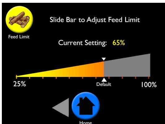
The Feed Limit screen allows you to adjust the amount of fuel being fed to the burn pot. The factory default for this is 65% which is best for most pellets. Adjustment may be needed based on fuel quality.
