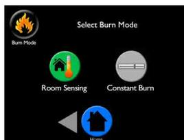
**Automatic and Constant Burn mode:** The unit will automatically ignite and will operate at your selected Constant Burn setting. The unit will not shut down unless the On/Off icon is touched or if the hopper runs out of fuel.
